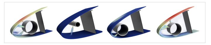
Figure 4: Improving the heat transfer performance of an aircraft ice protection system (courtesy: Honda Aircraft).
