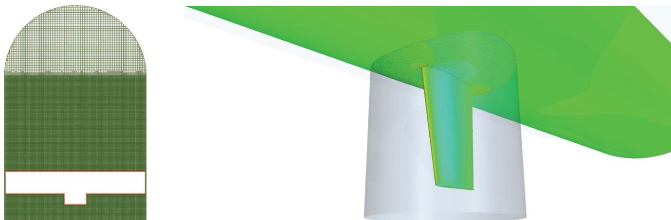
Figure 7: Overset topology options: piston (left) and direction (right).
